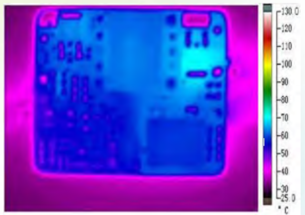
Figure 4: Thermal plot without airflow ( T_A = 25^\circ\text{C} ( 77^\circ\text{F} ); V_{in} = 48\text{ V} ; V_{out} = 12\text{ V} ; I_{out} = 2\text{ A} )
