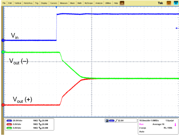
Figure 9: Startup from power on
