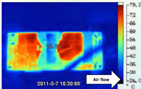
Figure 5: Thermal plot with airflow from V_{in} to V_{out} ( T_A = 25^\circ\text{C} ( 77^\circ\text{F} ); Airflow = 1 m/s (200 FLM); V_{in} = 48\text{ V} ; V_{out} = 3.3\text{ V} ; I_{out} = 15\text{ A} )
