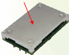
Figure 21: Thermal test point
