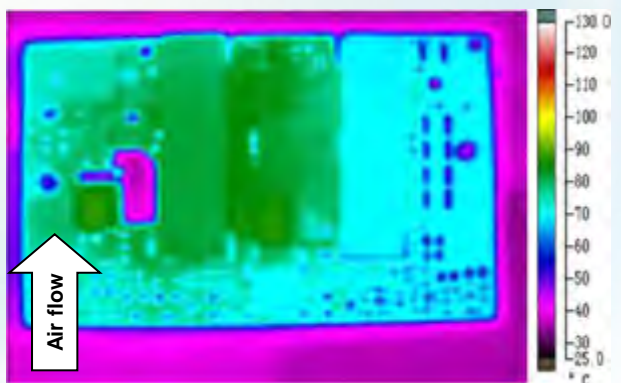
Figure 6: Thermal plot with airflow from V_{in}(-) to V_{in}(+) ( T_A = 25^\circ\text{C} ( 77^\circ\text{F} ); Airflow = 1 m/s (200 FLM); V_{in} = 48\text{ V} ; V_{out} = 24\text{ V} ; I_{out} = 3\text{ A} )
