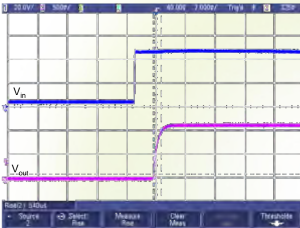
Figure 13: Startup by power on
