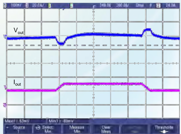
Figure 16: Output voltage dynamic response (Load: 50% - 75% - 50%, di/dt=0.1\text{ A}/\mu\text{s} )
