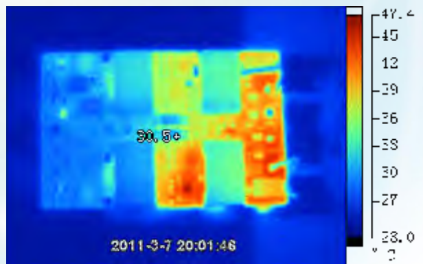
Figure 6: Thermal plot with airflow from V_{in}(-) to V_{in}(+) ( T_A = 25^\circ\text{C} ( 77^\circ\text{F} ); Airflow = 1 m/s (200 FLM); V_{in} = 48\text{ V} ; Full load)
