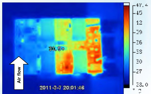
Figure 6: Thermal plot with airflow from V_{in}(-) to V_{in}(+) ( T_A = 25^\circ\text{C} ( 77^\circ\text{F} ); Airflow = 1\text{ m/s} ( 200\text{ FLM} ); V_{in} = 48\text{ V} ; Full load)
