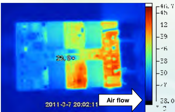
Figure 5: Thermal plot with airflow from V_{in} to V_{out} ( T_A = 25^\circ\text{C} ( 77^\circ\text{F} ); Airflow = 1\text{ m/s} ( 200\text{ FLM} ); V_{in} = 48\text{ V} ; Full load)
