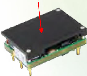
Figure 21: Thermal test point
