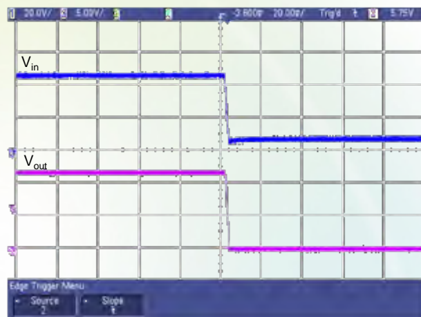
Figure 12: Shutdown by power off
