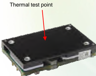
Figure 20: Thermal test point
